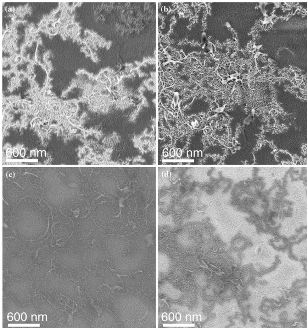
**Fig. 2** SEM images of CNTs on Au (10 nm)/glass substrate at **a** 1 kV, **b** 2 kV, **c** 5 kV, and **d** 10 kV
