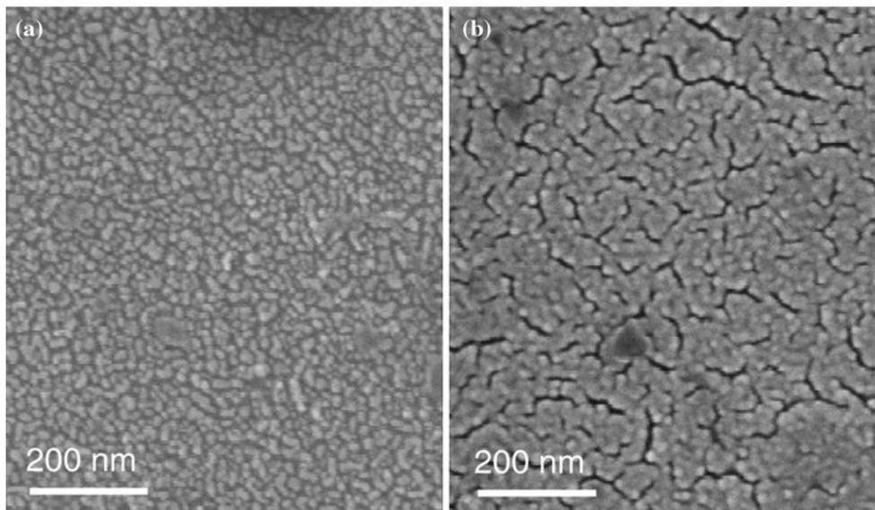
**Fig. 4** SEM image of **a** 10 nm and **b** 50 nm Au film on glass substrate
