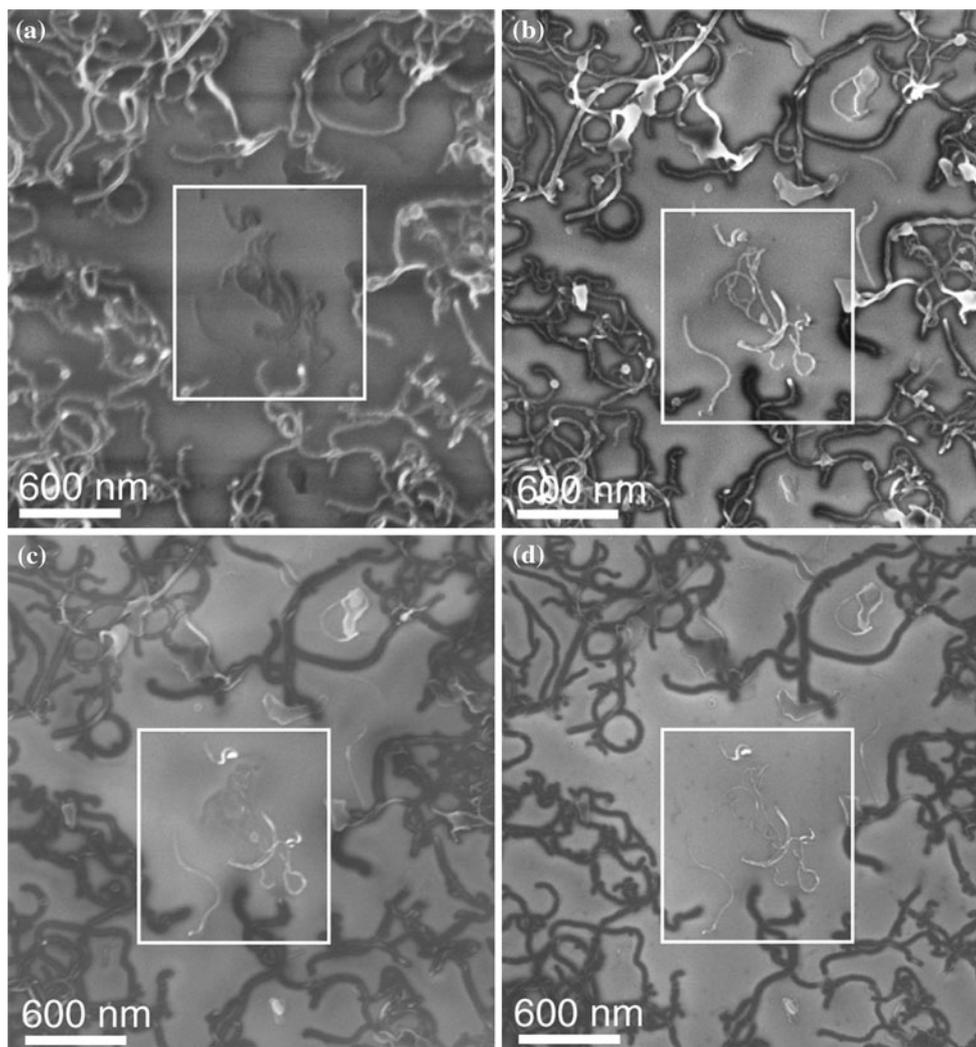
**Fig. 1** SEM images of CNTs on glass substrate at **a** 1 kV, **b** 2 kV, **c** 5 kV, and **d** 10 kV
