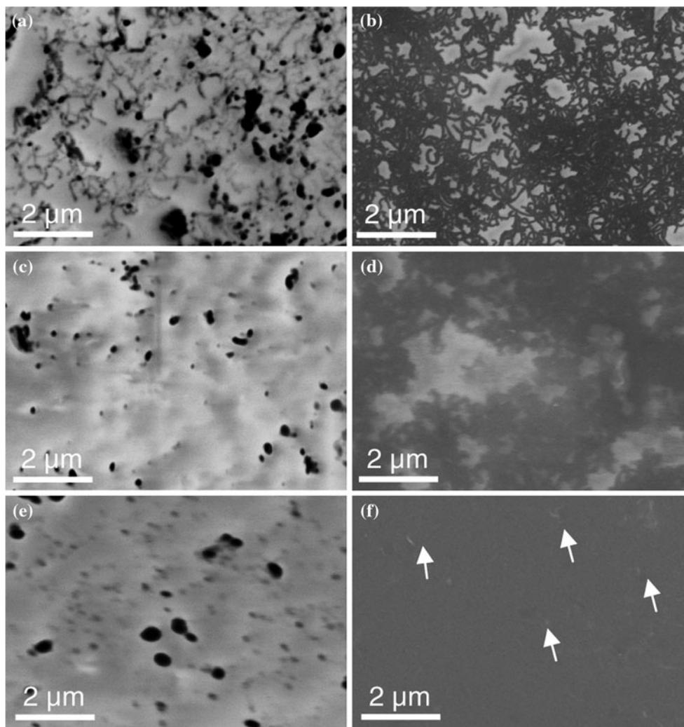
**Fig. 6** SEM images of CNTs on different substrates coated with a polystyrene film of 80 nm. On glass substrate at 1 and 10 kV (**a, b**), on Au (10 nm)/glass substrate at 1 and 10 kV (**c, d**), and on Au (50 nm)/glass substrate at 1 and 10 kV (**e, f**)
