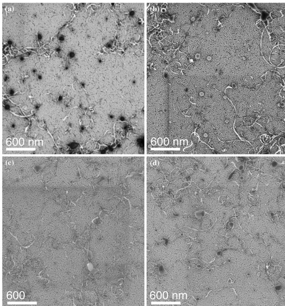
**Fig. 3** SEM images of CNTs on Au (50 nm)/glass substrate at **a** 1 kV, **b** 2 kV, **c** 5 kV, and **d** 10 kV
